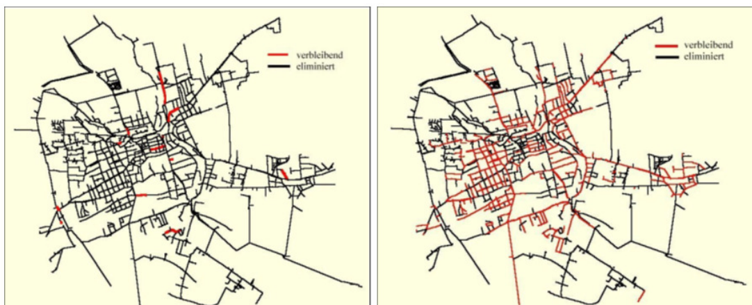
Renewal planning – Evaluation of acuteness and priorities of pipe replacement Pict. 1: short term replacement Pict. 2: medium term replacement
